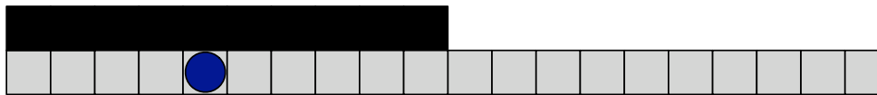
Figure 1. The Black and White world. The agent follows a random walk right and left, occasionally observing the color above it. The states wrap.
