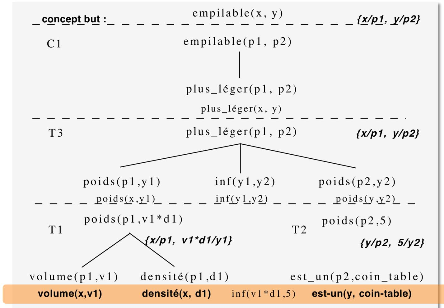
**Generalized search tree** resulting from **regression of the target concept in the proof tree** by computing at each step the most general literals allowing this step.
