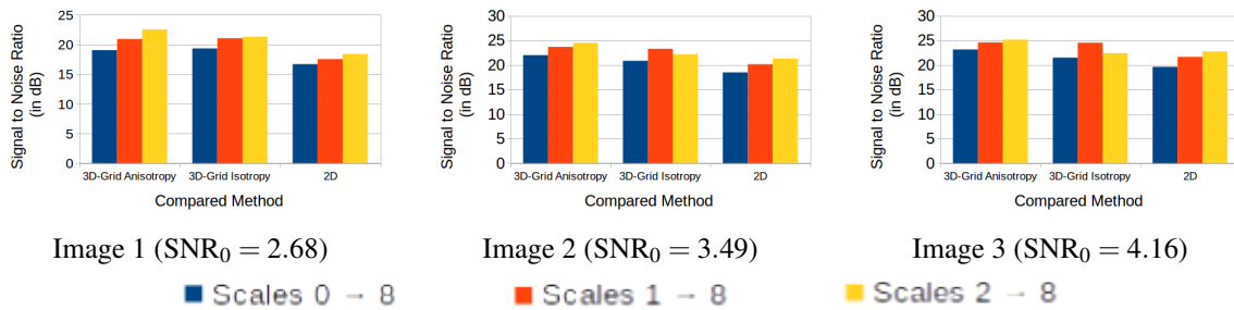
Figure 4: Signal-to-noise ratio of the output of the three denoising methods. From left to right: application to three different images. Inside each bar chart, from left to right: our 3D method with grid anisotropy, a 3D method without anisotropy, the 2D method. In blue/red/yellow: three different scale ranges.
